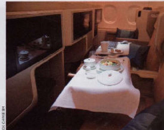
A pair of seats in New Business Class. Although similar to those on the Boeing 777-300ER, these are 4in (10cm) wider with greater pitch and have been re-contoured for greater comfort. The KrisWorld screens (above) are 15.4in (39cm) in width.
